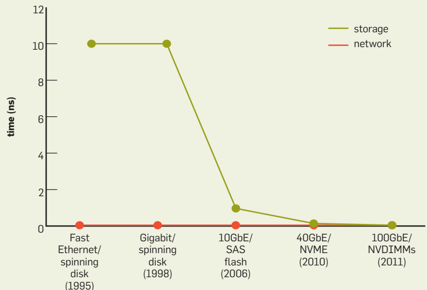
Figure 2. Progression in speed of SCMs compared to network adapters.
